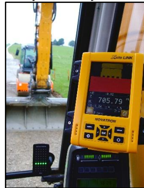
The control panel displays all current values and the green line on the panel shows the operator when he has reached the target depth
