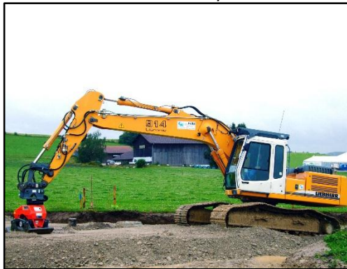
The vibrating plate compactor is also calibrated so that the operator can use it to read the current depth with the excavation system
