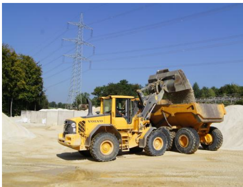
Loading the trucks, it is critical that the permissible total weight of the trucks
