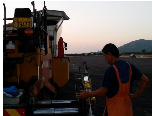
Thanks to the night-time design of the MOBA-matic II control panel, operating it in the dark is no problem
