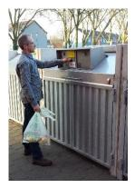
Using an RFID chip: the user is identified via the chip, the refuse container lock opens and the user can throw in his or her rubbish
