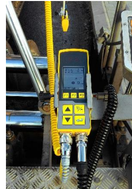
Control panel MOBA-matic II
