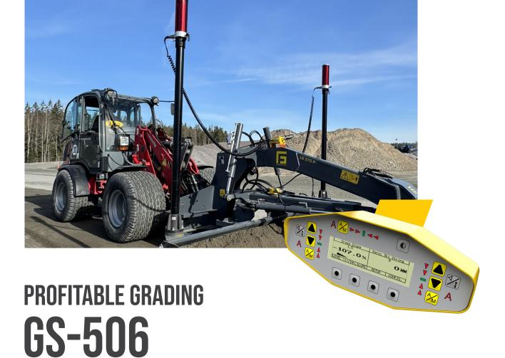
Whether for crawlers, graders, kilvers, or levelling blades, the 2D levelling system upgrades your machine with advanced height and inclination control. The coulter is fully automated, ensuring evenly distributed material and flawless flatness.
